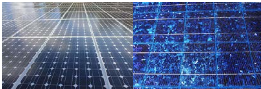
Figure 1. Monocrystalline cells (left) have a distinctive rounded geometric shape and appear smooth, while polycrystalline cells (right) are rectangular with a jagged internal structure. (DebbieMous, 2011; Andrewatla, 2007)
