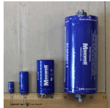
Figure 6. Pictured are four supercapacitors. From left to right they are, 5 F, 50 F, 350 F, and 3000 F.
