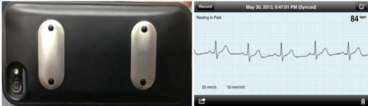
Figure 4. (Left) Commercial ECG screening device from Alivecor. (Right) Recorded ECG data using the Alivecor device
