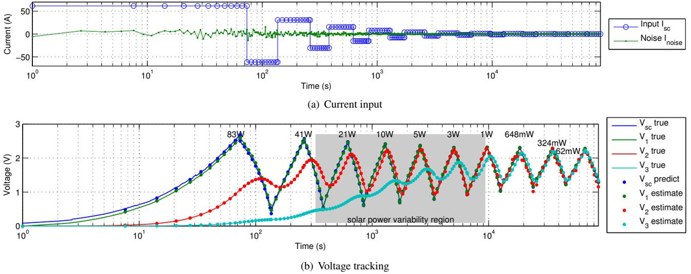
**Fig. 2.** The current (a), and voltage (b) charge-discharge profiles tests EKF state tracking over a range of power levels. The logarithmic scale shows cycles ranging from in duration from  $\sim 1$  minute to  $\sim 9$  hours.
